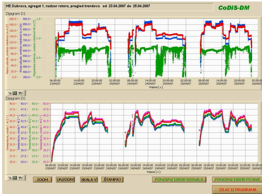
Fig. 3. Trending of electrical quantities (diagram D1: excitation current/voltage) and temperatures (diagram D2) on generator 1 in HPP Dubrava.
