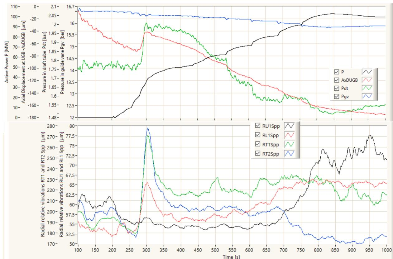
Fig. 8 – Static axial displacement (red), draft tube pressure (green), spiral case pressure (blue), active power (black) on top diagram. Radial relative shaft vibration p-p values at upper generator bearing (black), lower generator bearing (red), turbine bearing both directions (green and blue).
