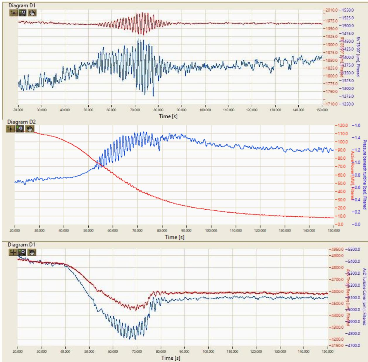
*Fig. 3 - Dynamic signal components during RLZ occurrence, load reduction operation – Radial relative shaft vibrations on generator (blue) and turbine (red) bearing on top diagram, active power (red) and static draft tube pressure (blue) on middle diagram, axial displacements on top of generator (red) and turbine cover (blue) on bottom diagram*
