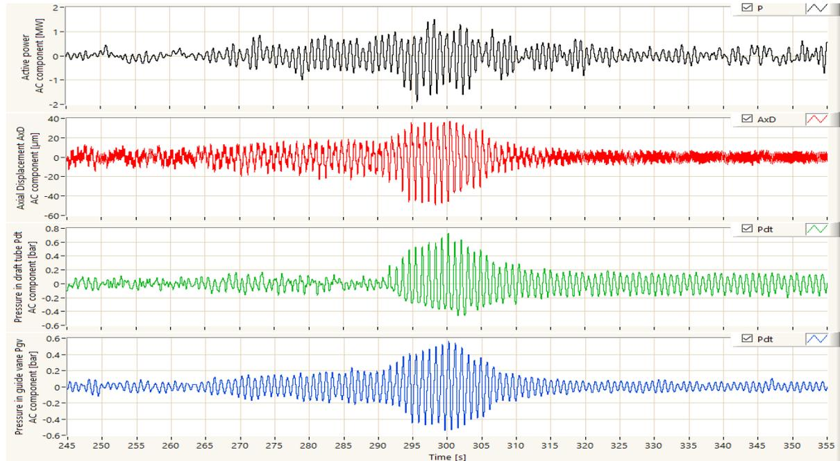
*Fig. 7 – Bandpass (0.1 to 1 Hz) filtered waveforms of active power (black) on top diagram, axial displacement on top of generator (red), draft tube pressure (green), spiral case pressure (blue), recorded during load increase at 45 MW load*
