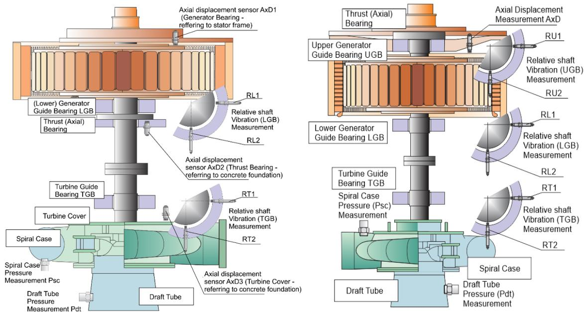
Figure 1 – Basic design, bearing disposition and measurement sensors layout for analyzed units, left side refers to Unit 1 and Unit 2, right side refers to Unit 3
