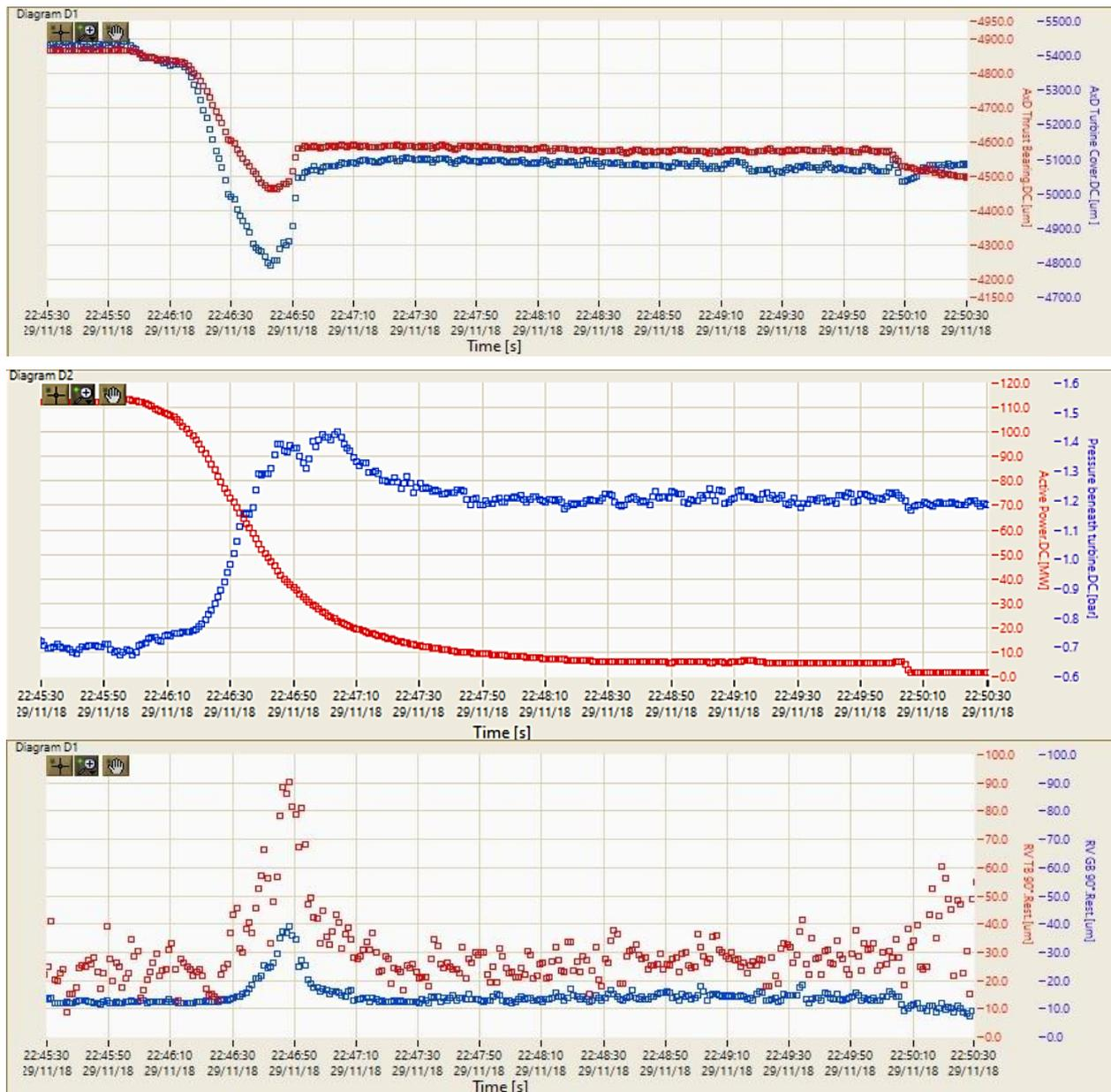
Figure 2 -Static axial displacements on top of the generator (top diagram, red color), on turbine over (top diagram, blue color), active power reduction 120 to 10 MW (middle, red color), static pressure in draft tube (middle, blue color), relative shaft vibration REST value (turbine guide bearing - red color, lower generator bearing – blue color)
