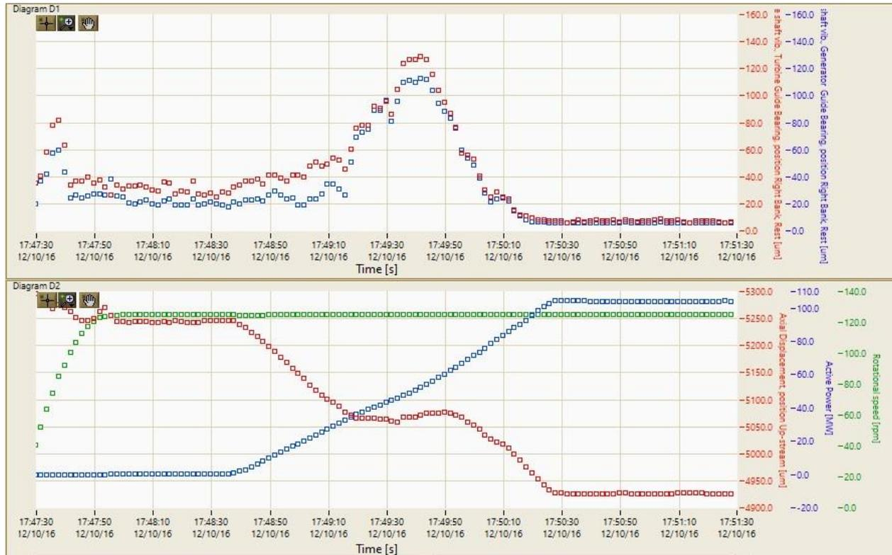
Fig. 5 – Radial relative shaft vibrations REST value on generator (blue) and turbine (red) bearing on top diagram, active power ascending from 0 to 108 MW (blue), axial displacement of rotor referred to axial bearing bracket (red) and rotational speed (green) on bottom diagram
