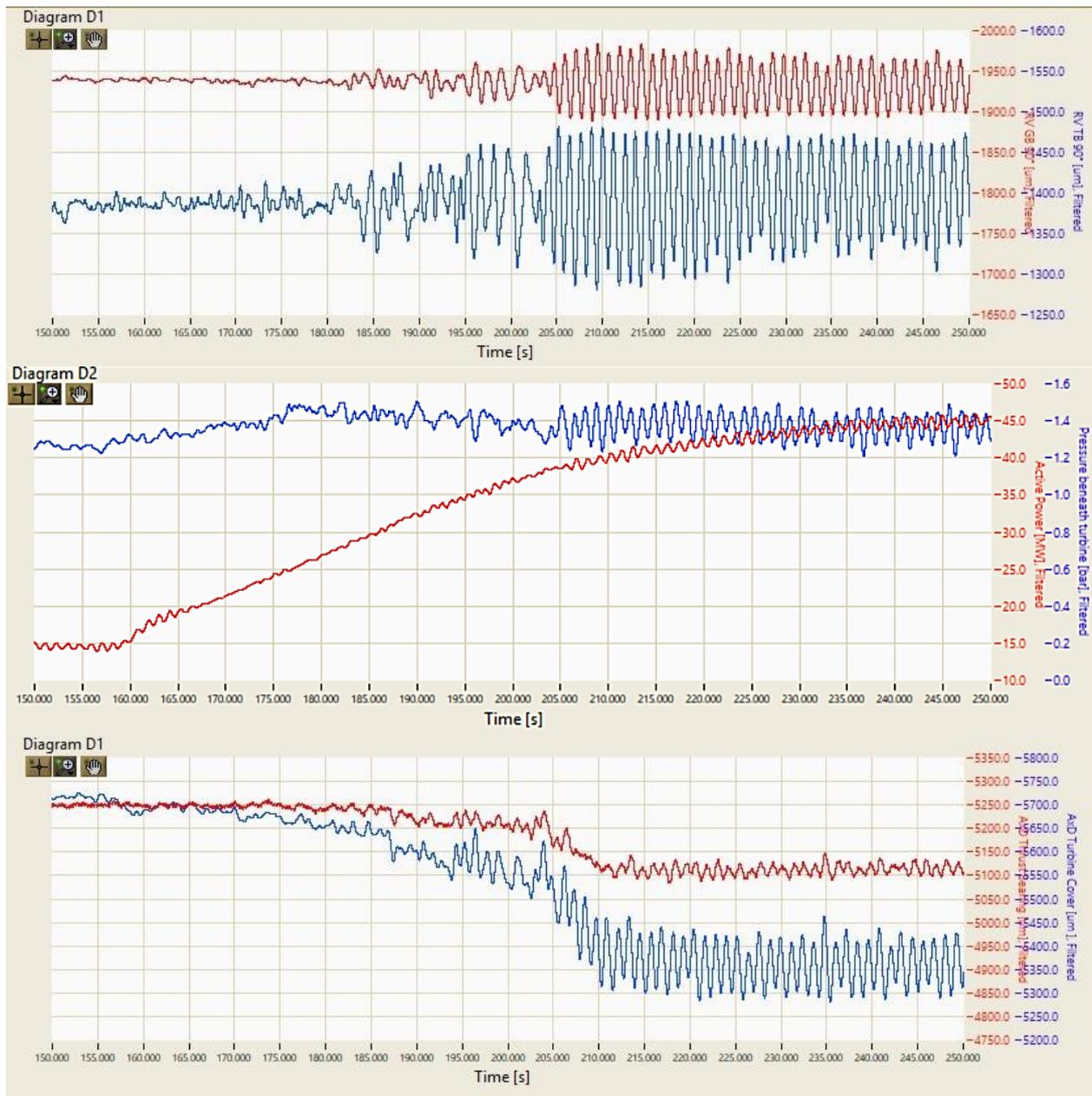
Fig. 4 - Dynamic signal Waveforms during RLZ occurrence, load increase operation – Radial relative shaft vibrations on generator (blue) and turbine (red) bearing on top diagram, active power (red) and static draft tube pressure (blue) on middle diagram, axial displacements on top of generator (red) and turbine cover (blue) on bottom diagram
