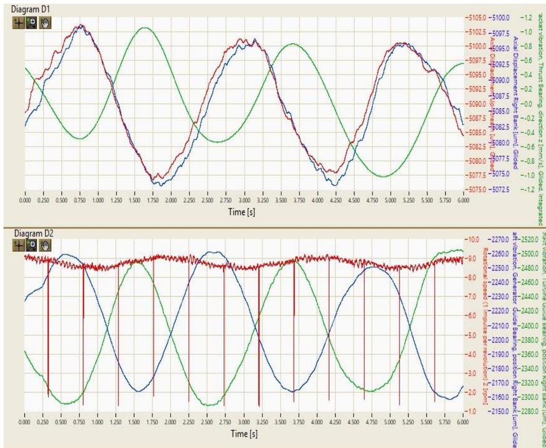
Fig. 6 – Rotor axial displacement (red and blue), axial bearing bracket displacement (green) on top diagram, relative radial shaft vibrations on generator (blue) and turbine (green) bearing and diagnostic trigger signal (red) on bottom diagram. Data recorded on 45 MW (RLZ)
