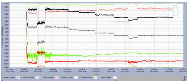
excitation on the vibrations on the TGB. It can also be seen that the vibrations decreased on LGB – lower guide bearing (red) from ~100  $\mu\text{m}$  to ~10  $\mu\text{m}$ . Vibrations on the UGB – upper guide bearing (black) appear to not change significantly (in amplitude). But when looking at the phases of the 1x harmonic, it can be clearly seen that there is a significant load dependence on the UGB. On the LGB and UGB, these
