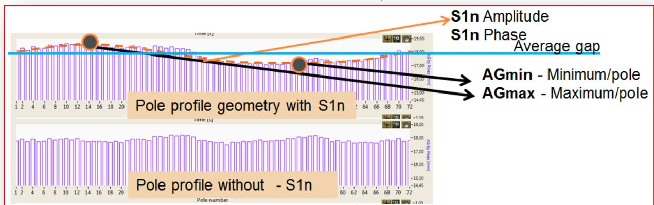
Fig 1.- Compensation of dynamic part of the signal from geometry of rotor body
